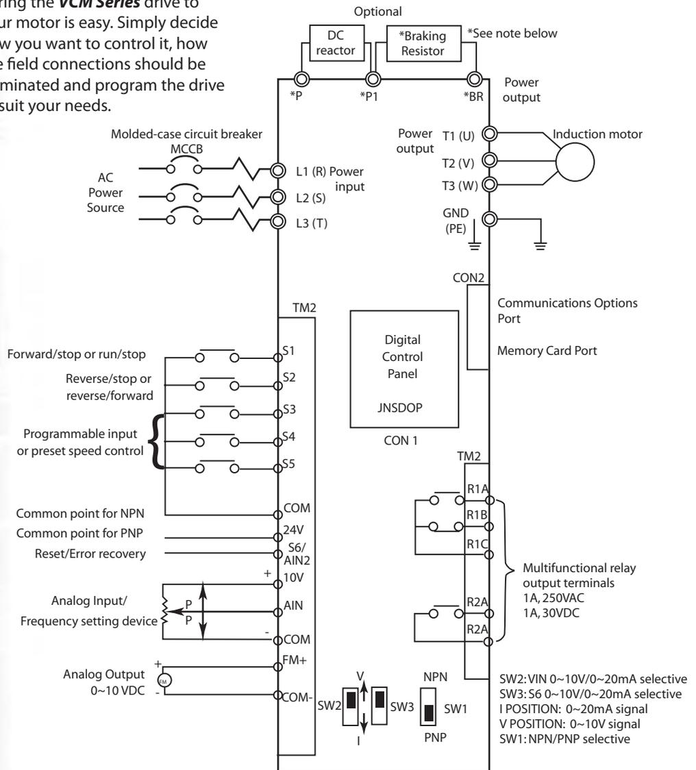
\* Note: Diagram applies to models rated up to 10HP at 240V and 15HP at 480V. Contact factory for power schematic for larger sizes.
