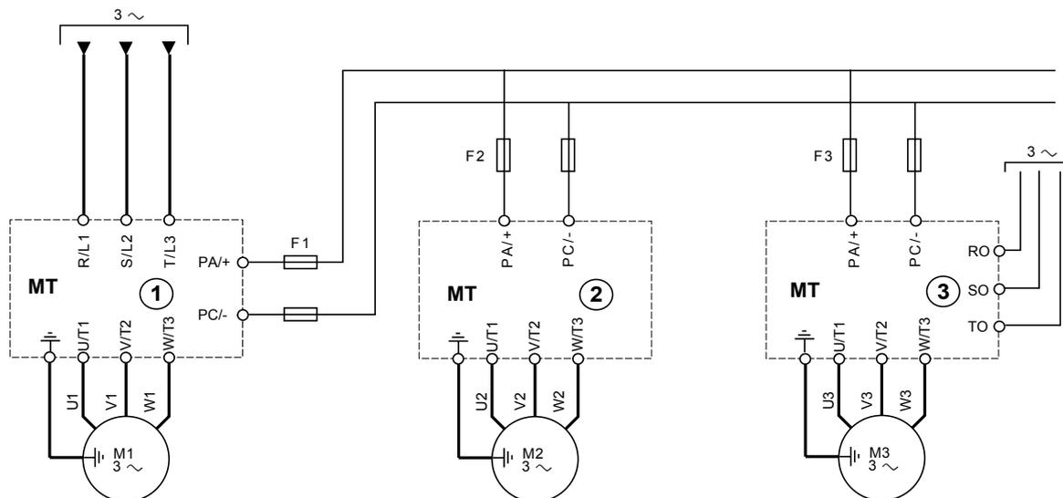
Drives ② and ③ powered by their DC buses only do not need to have a DC choke (catalog number MT).
