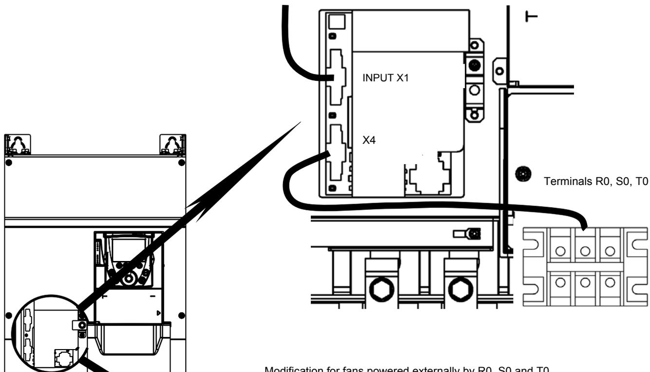
Modification for fans powered externally by R0, S0 and T0
