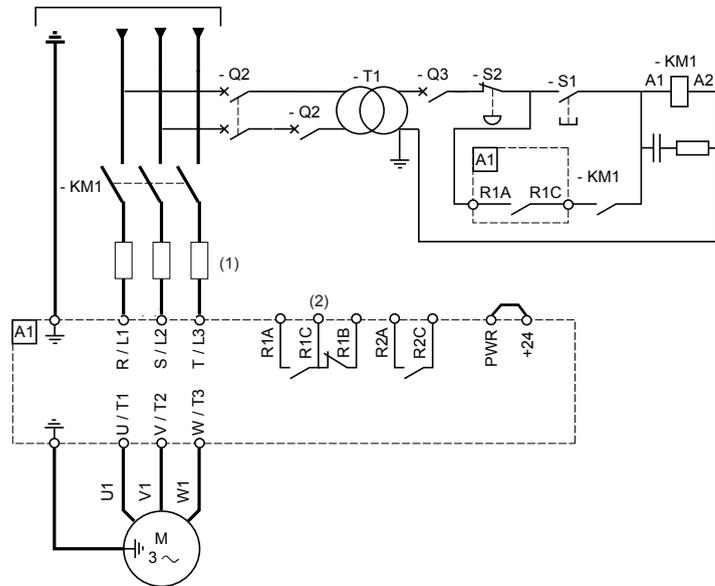
Diagram with disconnect switch
