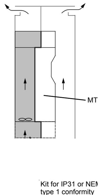
Several methods of evacuation are possible. The following is a proposed method for IP23 or IP54 mounting.
