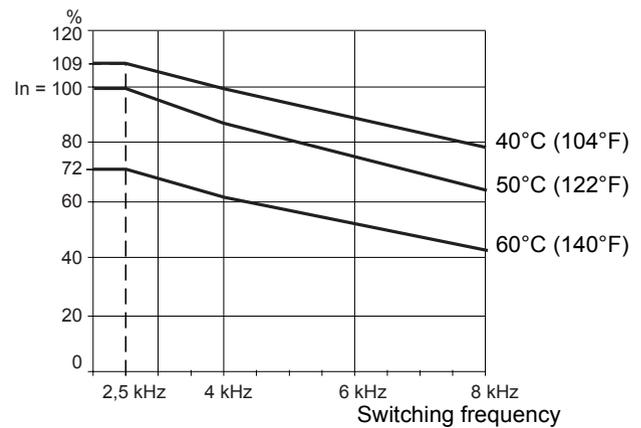
For intermediate temperatures (e.g. 55°C (131°F)), interpolate between 2 curves.
